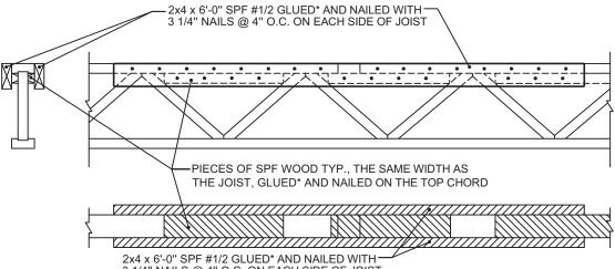
2x4 x 6'-0" SPF #1/2 GLUED\* AND NAILED WITH- 3 1/4" NAILS @ 4" O.C. ON EACH SIDE OF JOIST
