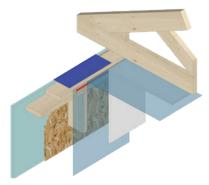
Air barrier continuity at wall-to-roof junction transferred through interior vapour barrier.
