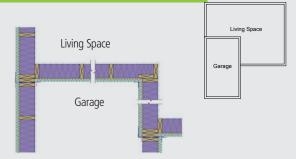
Exterior walls of heated garages must be built like other exterior walls.
